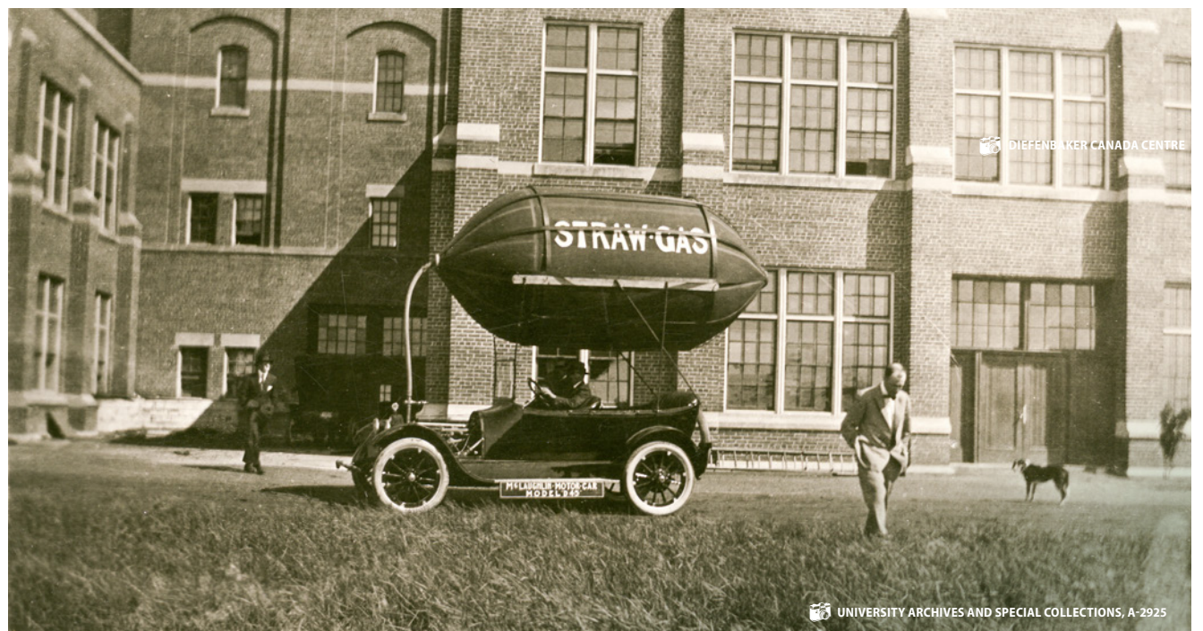
USask's unique experimental straw fuel car—the McLaughlin Motor Car Model D45—on campus in 1918.
