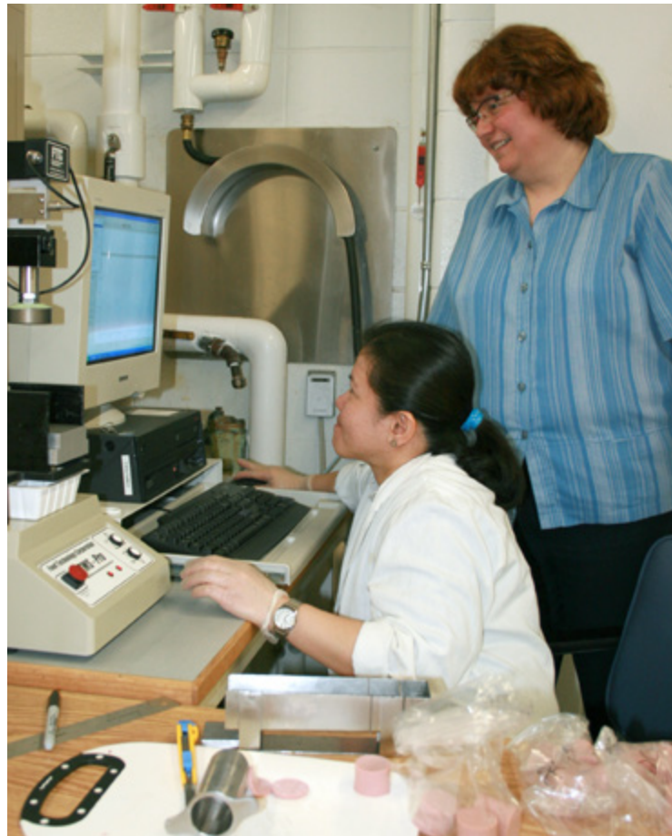
Phyllis Shand (right) and research technologist Marilyn Edrosolam test compression and springiness of low-sodium bologna samples.
