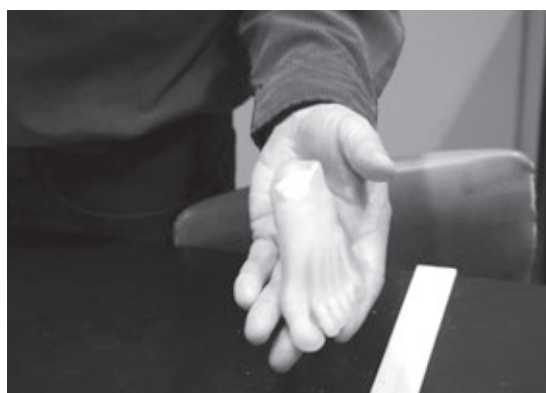
A human foot displaying bone structure shows off the advantages of 3-D printing in two materials at once.
