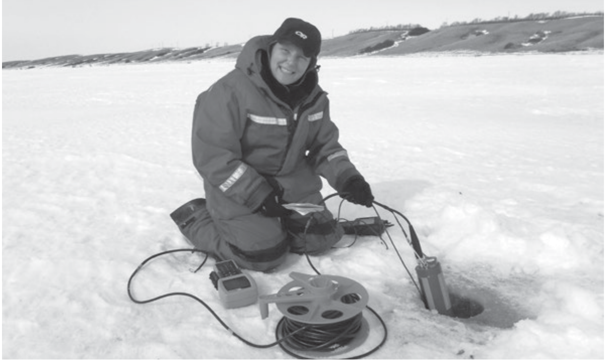
Rebecca North measures winter oxygen levels and water temperature at Lake Diefenbaker.
